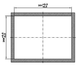
Necessary opening size (± 0.5): Width: 351.0 mm / Height: 266.0 mm
