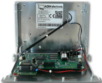
The TFT-Industrial-Monitor is a modern concept to replace old or defective CRTs mounted in control units of Bosch. All units are Made in Germany, using only high quality components. A mechanic housing, similar to the original unit, makes it easy to exchange in just a few minutes. The new display is plug&play 100% compatible to the Bosch equipment.
